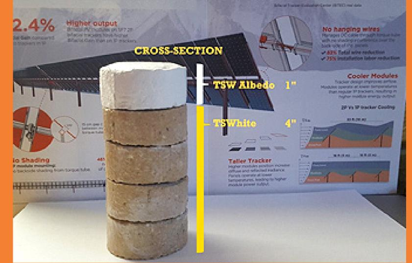
The higher the albedo of the surface under your bifacial panel, the more gain you can realize from your bifacial panel. The darker the surface under your bifacial panel, you will not be able to realize the complete xx% UNLESS you have the albedo of smooth fresh fallen snow which is 0.80 to 0.90. We believe this soil stabilizer can give the ground a permanent, consistent and highly reflective surface.
